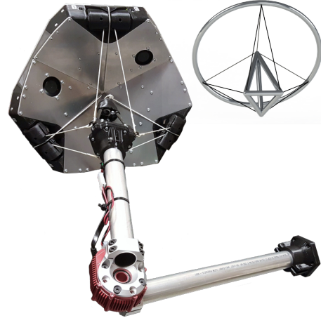
Fig. 1. A picture of our 3 DOF Joint within a robotic arm assembly. On the top right is a simplified model of our joint shown in the same orientation, showing the connectivity of the topology for clarification.
