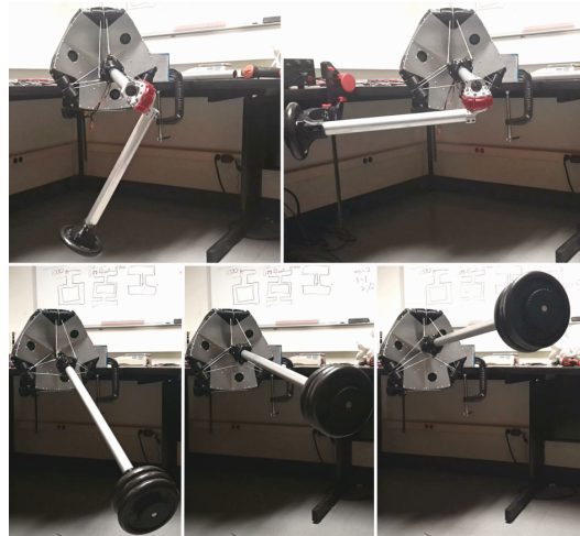
Fig. 11. The joint was affixed with a HEBI X-series actuator to serve as an elbow with a 1.2 kg proof mass attached (above). The arm was then held up by our joint while the elbow was held at a right angle. Our joint was then used to lift the proof mass demonstrating its ability to apply a torsional moment of 6 Newton-meters. Next the joint was affixed with a 95cm rigid arm (below) and a proof mass of 7 kilograms. In this configuration the prototype was able to lift the mass with a maximum cable-tension of 310 Newtons to apply a 65 Newton-meter torque.
