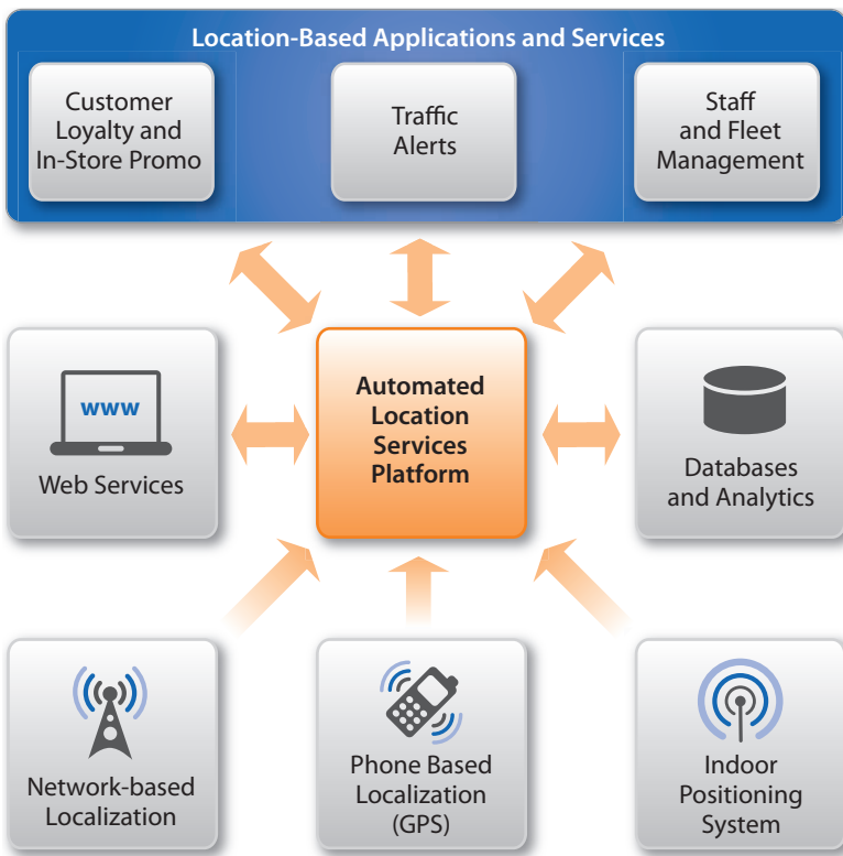
Figure 2. Examples of the many systems which must be integrated by the Automated Location Services Platform in order to support a wide range of location based applications and services.
