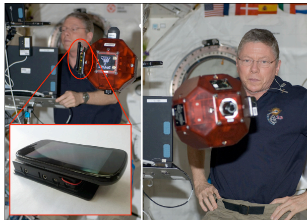
Figure 10. Astronaut Mike Fossum testing Smart SPHERES. The Smartphone is shown in the inset (left). (NASA ISS029-E-036493 / -036497)
