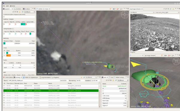
Figure 13. The Visual Environment for Robotic Virtual Exploration (VERVE) is an interactive 3D user interface for monitoring robot operations.
