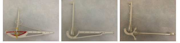
Fig. 8. Three iterations of passive tensegrity elbow joints. These prototypes demonstrate the flexibility and compliance of the tensegrity elbow without using motors.
