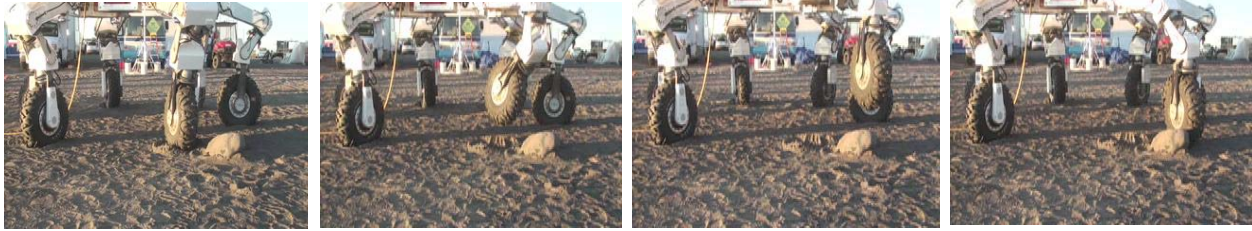
Figure 11. ATHLETE taking a step over a rock -- motion planned by the Footfall Planner Software
