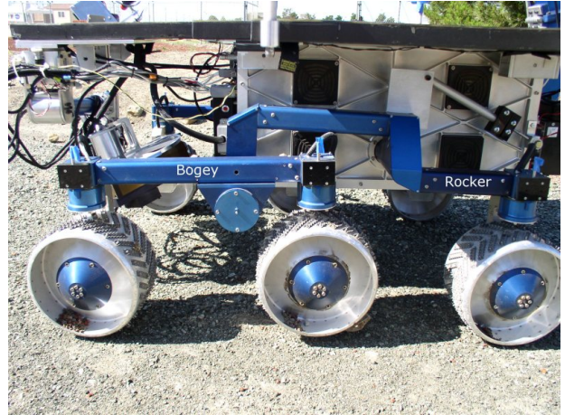
Figure 3. The suspension on the K-9 rover. The front of the rover is on the left, with the first two wheels attached to the bogey, which is in turn attached to the rocker, and then to the rover chassis.
