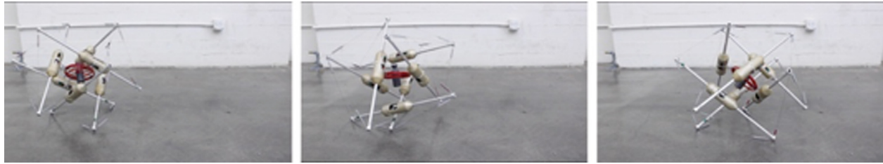
Fig. 17 TT-3 performs straight line walk while carrying a center payload
