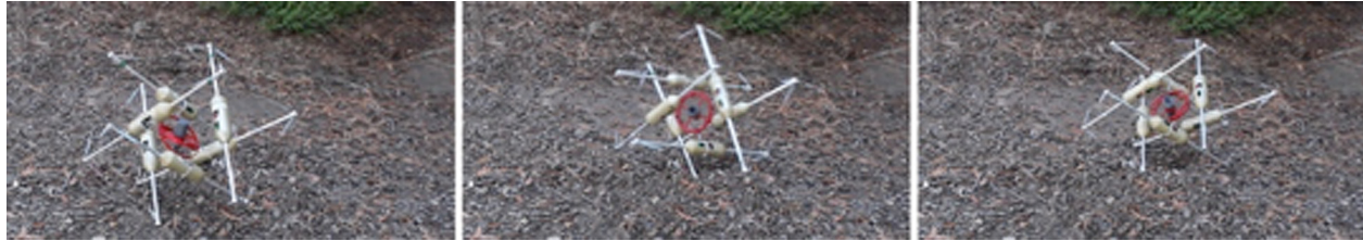
Fig. 18 TT-3 performs straight line walk on an uneven outdoor terrain
