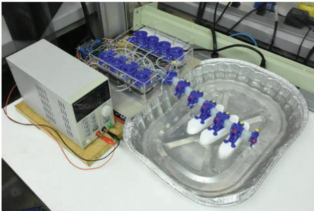
**FIG. 11.** Experimental setup with spine floating in water bath. Color images available online at [www.liebertpub.com/soro](http://www.liebertpub.com/soro)
